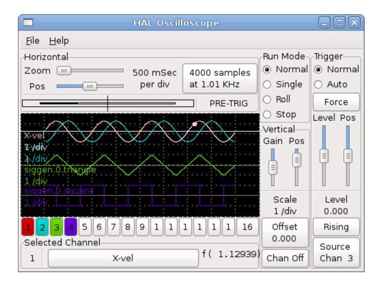
Figure 2.11: Waveforms with Triggering
